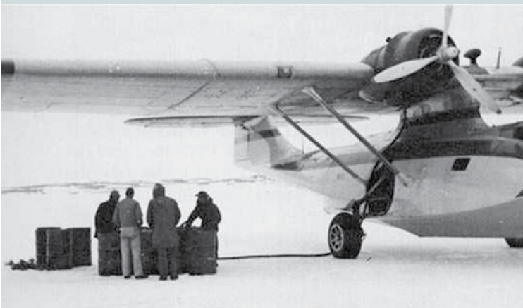
A Canso "Tanker" at Fergusson Lake. Cansos routinely flew in 700 gallons of diesel or avgas using one of the two big wing tanks. (Larry Milberry, 1985)
